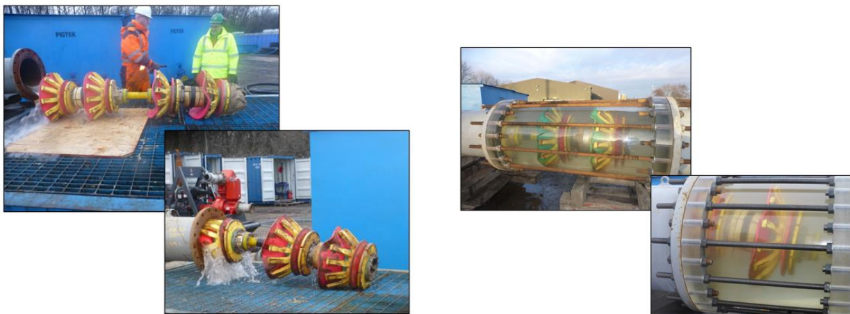
Figure 15 - 16/24E wax removal / compression test / passing through 24” & 34” acrylic spools.
