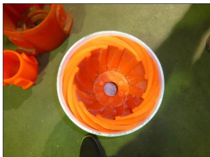
A typical Dual Diameter Pig Cup in compressed position
