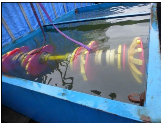
Figure 14 - 16/24E Neutral buoyancy check.
