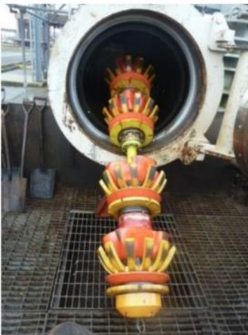
Figure 16 - 16/24E received at Teesside 34" pig receiver.
